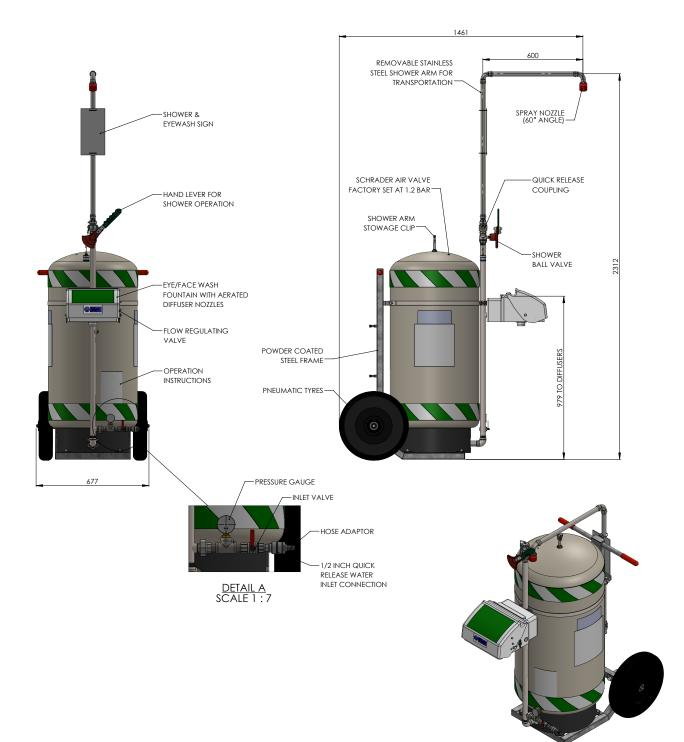
ISOMETRIC VIEW (SHOWER ARM ATTACHED TO FRAME WHEN TRANSPORTING
