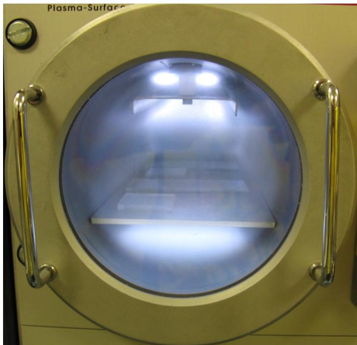
Figure 4.5: Glass and PDMS samples undergoing oxygen plasma exposure.
